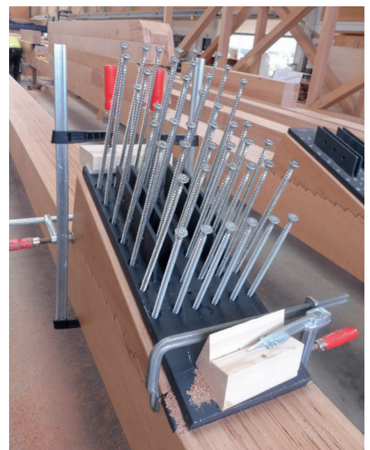
SWG production hall – Lattice girders connection with 12 mm full thread screws
